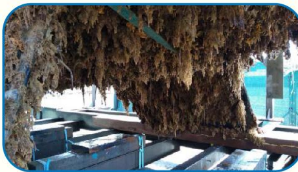
Thick biofouling – including unwanted Mediterranean fanworm – covering the hull of a vessel ordered out of the water at Mangonui for cleaning.
