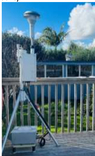
PM 10 monitor installed in Tikipunga
