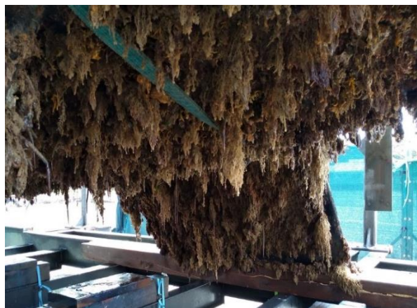
Thick biofouling – including unwanted Mediterranean fanworm – covering the hull of a vessel recently ordered out of the water at Mangonui for cleaning.
