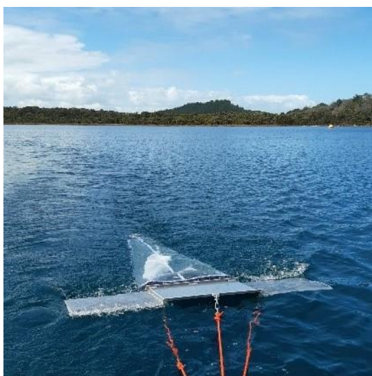
Trawling plankton in Lake Taharoa for microplastic sampling
