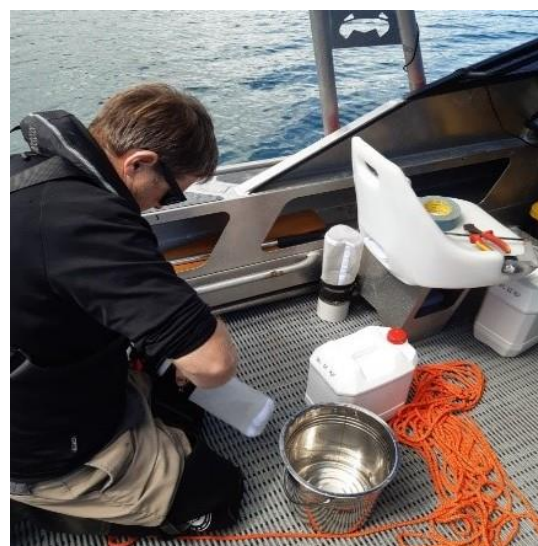
Filtering the water sample from the plankton net
