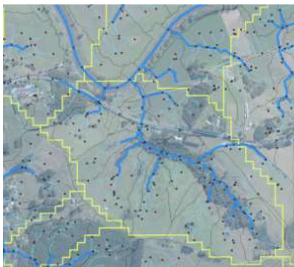
Figure 1. An example snapshot of DRN catchments (dark grey lines) with river lines at 2ha (dark blue), and 0.2 ha (light blue) scales in Tangiterōria. Dark brown dots indicate start and end points of each river segment. The yellow jagged lines are currently available coarser catchments (i.e., NIWA river network model).
