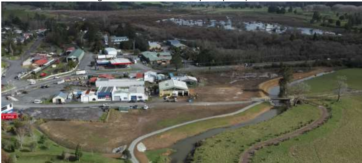
Drone shot looking downstream at the final form of the deflection bank on the left hand bank of the Waiomio River
