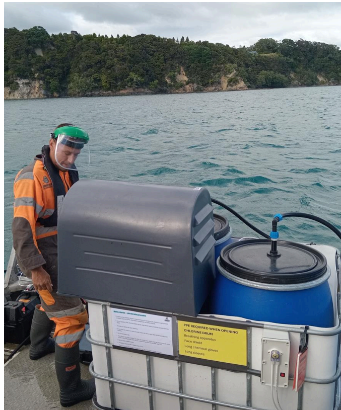
The equipment on board the accompanying vessel to deliver chlorine to treatment area. Photo: Commercial Dive Specialists.
