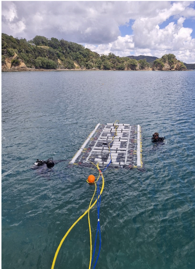
Advanced Aquarium Technologies Ltd test the UV-C treatment panels in the waters of Omakiwi Cove, Bay of Islands.
