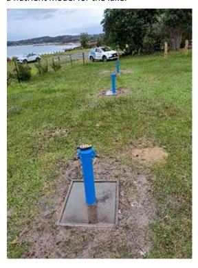
Photo left: show banks of Lake Ngatu – critical pieces of infrastructure that were recently installed to monitor nutrients, such as phosphate and nitrogen, in the lake system.
