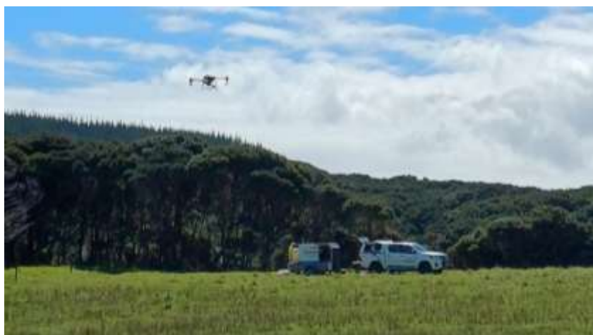
A drone in operation above Lake Waikanae in the Far North, applying herbicide to control the invasive lake plant hornwort.
