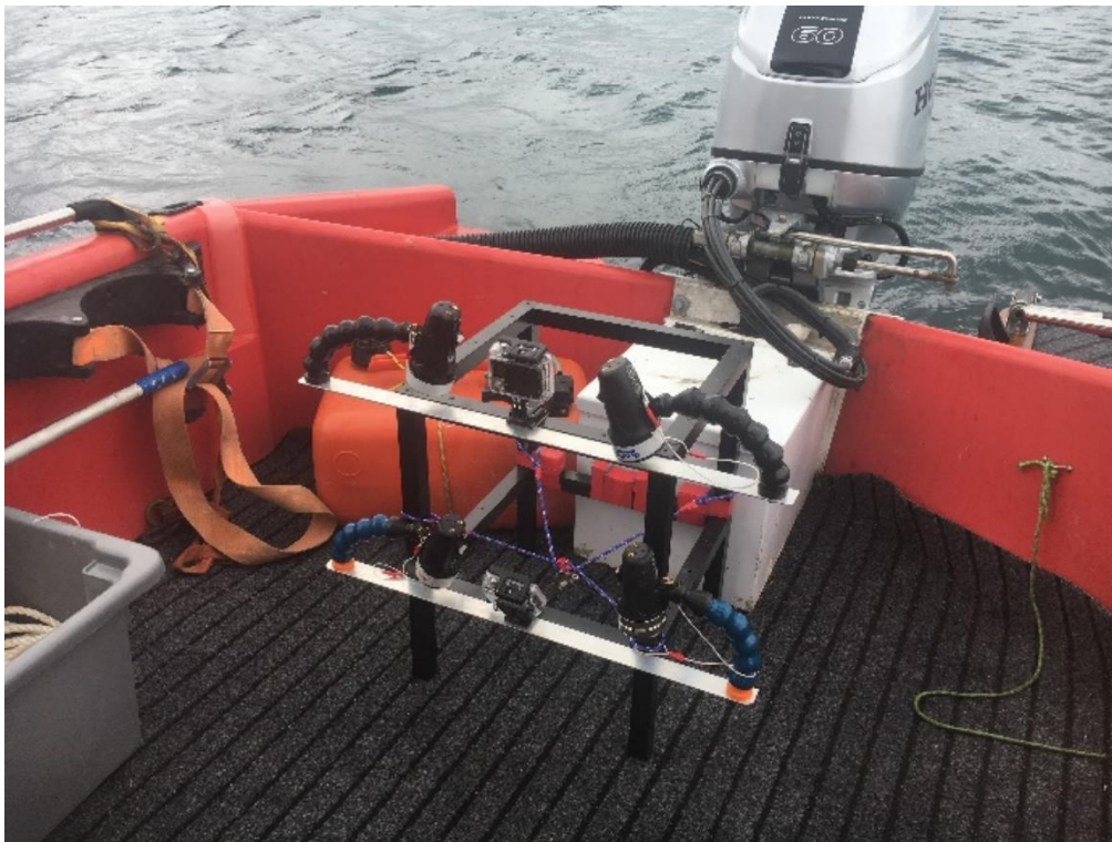
Plate 3. Drop camera set up with two GoPros and underwater lighting used in the Ipipiri survey.
