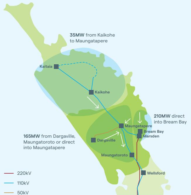
Figure 8: Illustration of existing network export capacity
